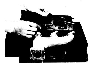
How to check cylinder head surface
