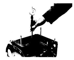
Measuring points of cylinder liner
